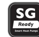
SG-Ready is a defined standard by BWP\*\*\*, which makes it possible that the device can be integrated into a smart grid. Heat pumps, which are equipped with the SG-Ready Label, can receive signals from the power grid (and e.g. also from PV systems) about the available (unused renewable) energy (from wind, sun & water). Fujitsu General provides the SG-Ready compatibility to all new Heat Pumps series.
